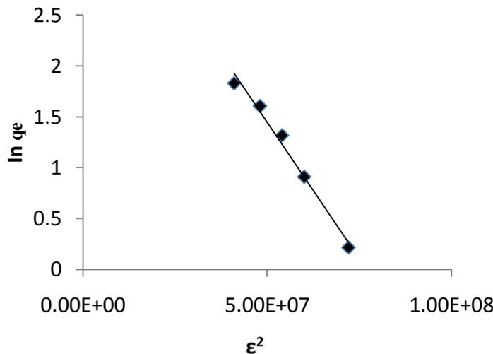
Figure 8: Dubinin-Radushkevich plot for the adsorption of MB
