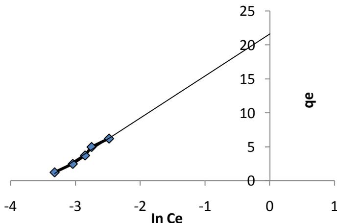
**Figure 6: Temkin isotherm plots for adsorption of MB by AC at 30°C.**
