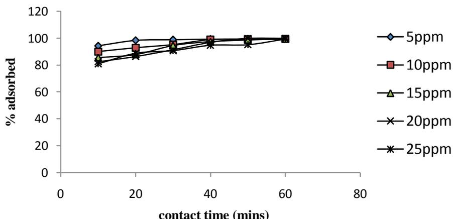
**Figure 4: Effect of contact time and initial conc on adsorption of MB onto AC.**
