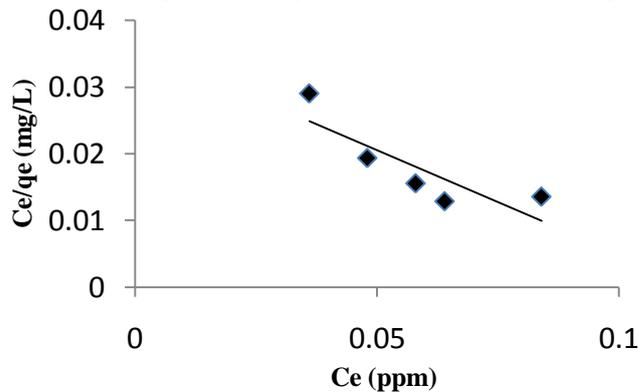
Figure 5: Langmuir isotherm for the adsorption of MB by the AC at 30°C
