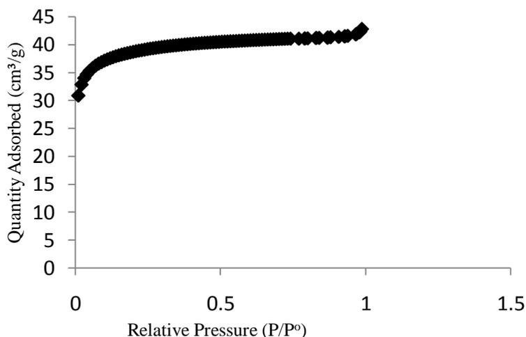
Figure 2: Nitrogen gas adsorption isotherm for the sample at 77 K.
