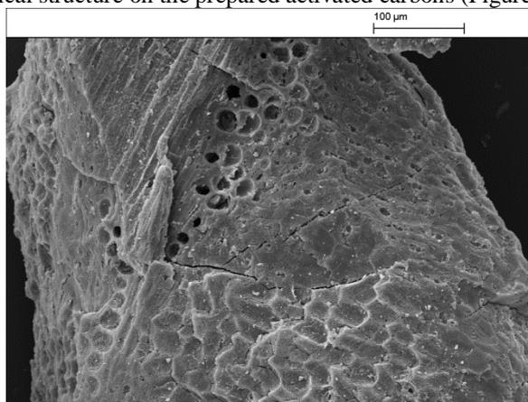
Figure 1: SEM of the prepared Activated sample
