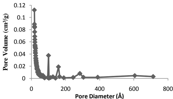
Figure 3: Pore size distribution of the sample
